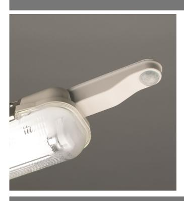
The EBMPIR-MB-PRM-110 miniature PIR (passive infrared) presence detector provides automatic control of lighting loads with optional manual control using an infrared handset. It is specifically designed for mounting onto a batten style luminaire that is powered by a 110V supply.
